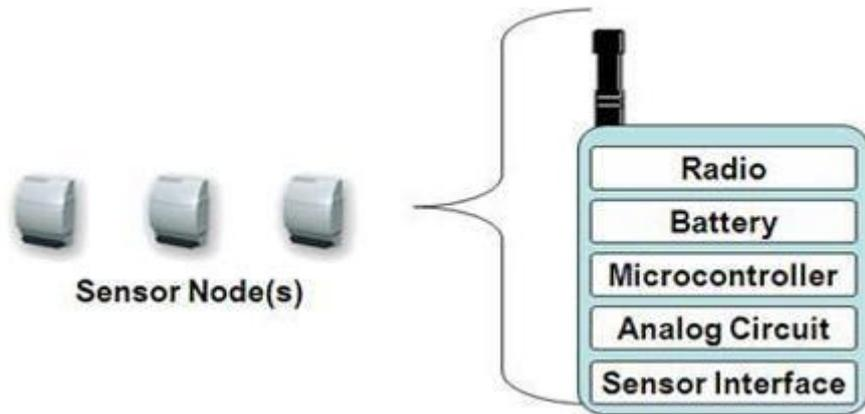
**Figure 3.** Components of a Wireless Sensor Node
