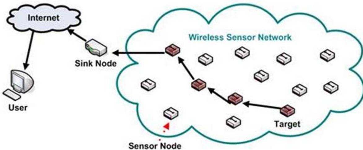
**Figure 1.** General Wireless Sensor Model
