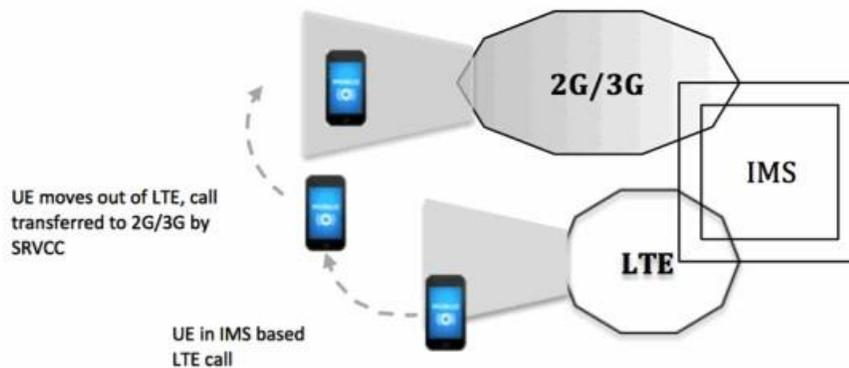
**Figure 8 Seamless handover procedure**
