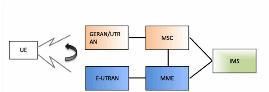
Figure 7 The SRVCC Architecture
