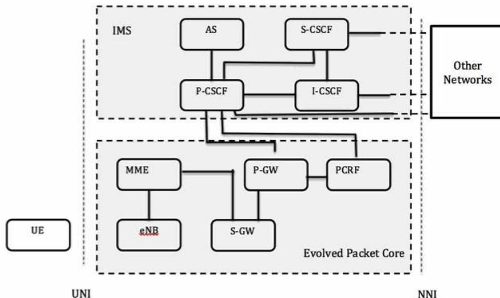
Figure 6 The GSMA VoLTE Architecture
