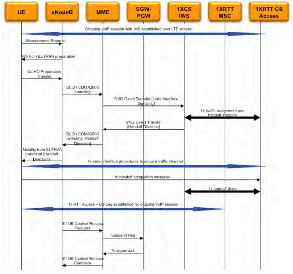
Figure 4. SRVCC from LTE to 1x CS Voice System
