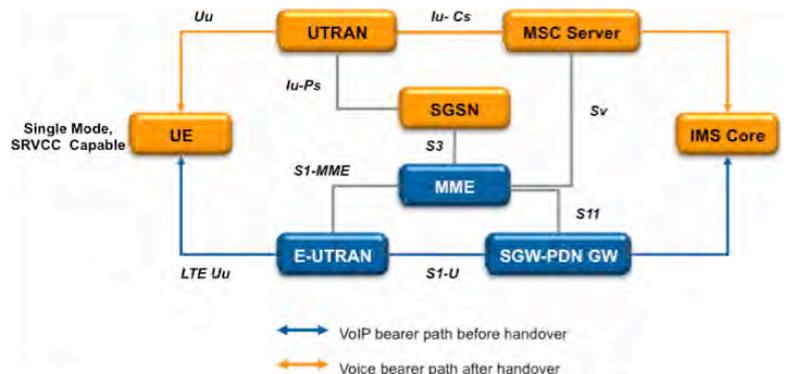
Figure 2. EPS Reference Architecture for SRVCC to UTRAN as Destination Network
