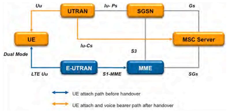
**Figure 1.** EPS Reference Architecture for CSFB with UTRAN as Destination Network
