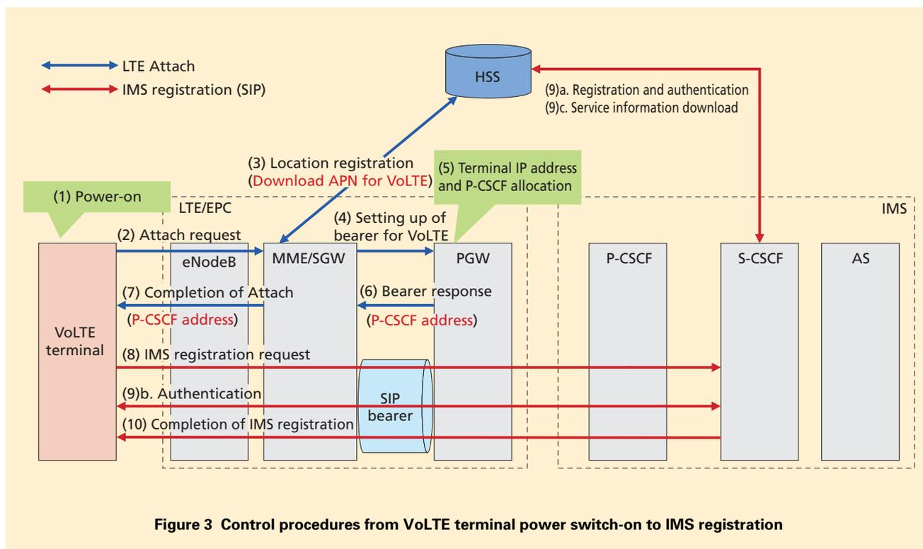
Figure 3 Control procedures from VoLTE terminal power switch-on to IMS registration
