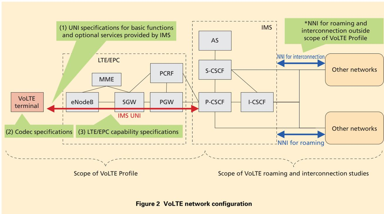
Figure 2 VoLTE network configuration
