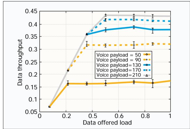
■ Figure 16. Effect of  $1_{\text{voice}}$  on data throughput.
