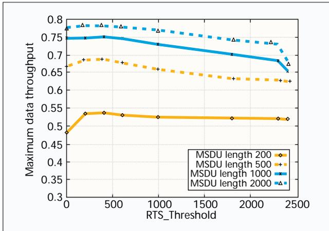
■ Figure 12. *RTS\_Threshold effects on data throughput.*
