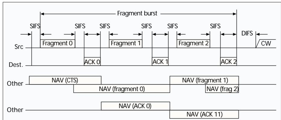
■ Figure 7. Transmission of a fragmented MPDU.
