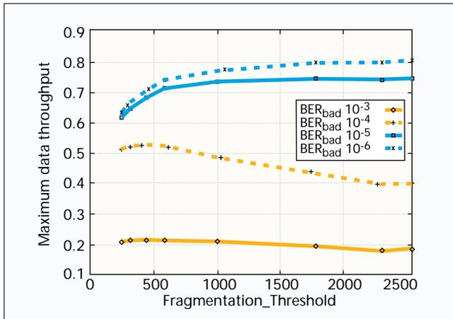
■ Figure 13. *Fragmentation\_Threshold effects on data throughput.*
