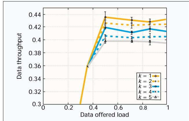
■ Figure 17. Data throughput vs. offered load for several values of  $k$ .
