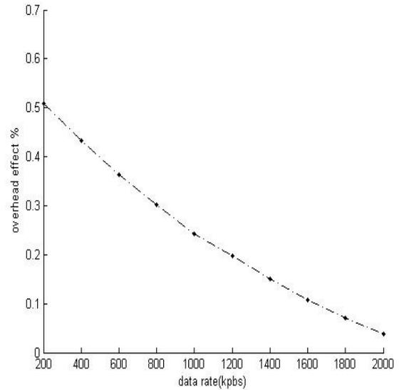
Fig. 7 The effect of overhead versus data rate
