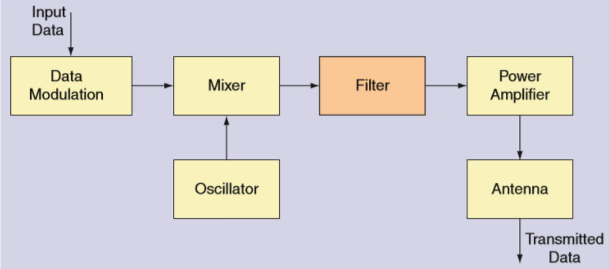
**Fig. 1** Block diagram of a typical a narrowband Transmitter
