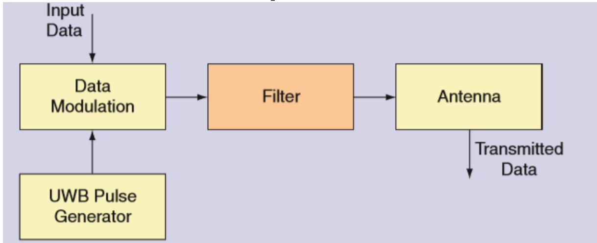
**Fig. 2** Block diagram of a typical UWB Transmitter
