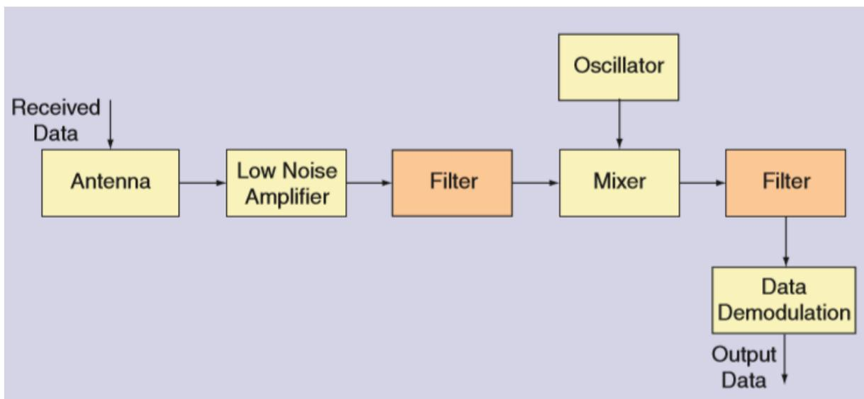
**Fig. 3** Block diagram of a typical a narrowband Receiver
