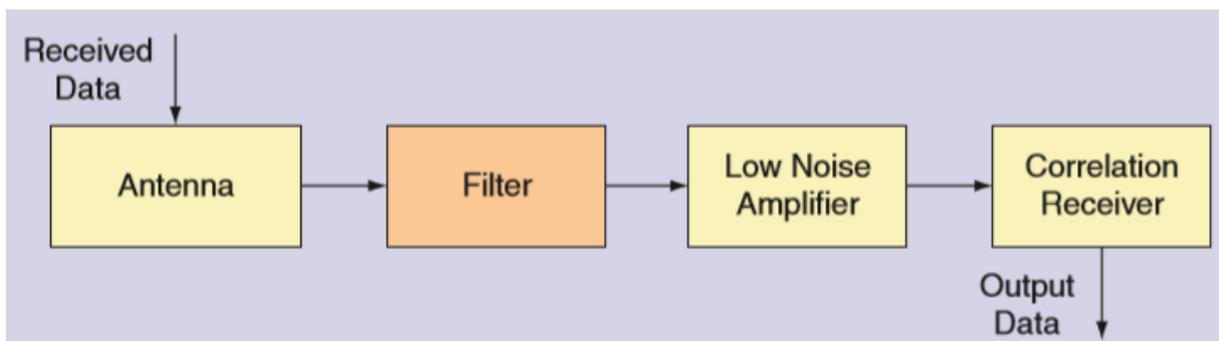
**Fig. 4** Block diagram of a typical UWB Receiver
